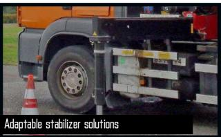
The stabilizer legs of the crane are to ensure stability - however they still have to be sturdy, easy to handle and must not take up too much space when not in use. Therefore you can choose between fixed stabilizer legs, manual swing-up stabilizer legs to 180° with gas spring or fully hydraulic swing-up stabilizer legs to 180°. Stabilizer beams can be freely selected as hydraulically extensible or manually extensible and also in connection with the sophisticated EVS stability monitoring system.
