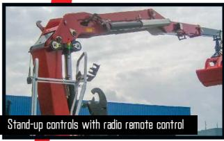
With stand-up control and radio remote controls the crane operator has an increased overview of the crane movements. The remote control is placed in a bracket on the stand-up platform where it is fixed whilst operating the crane. The crane operator is protected by the HSL or HSL-E safety system which prevents the crane from hitting the operator on the stand-up platform.
